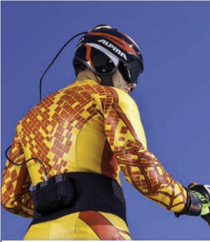
▲ STEALTH mounted on stretchable belt and helmet-mounted GNSS antenna.
